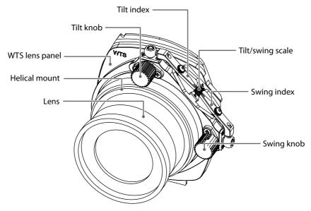
lock, where the drive knobs become slightly loose by purpose. To apply tilt only use tilt knob, to apply swing only use swing knob. When needed, a combination of both can be applied.
