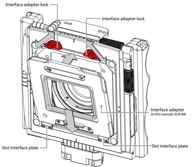
*Please note: the image shows the WRS-1200 body which features the same mounting system as the WRS-5000. All interface plates are interchangeable.*
