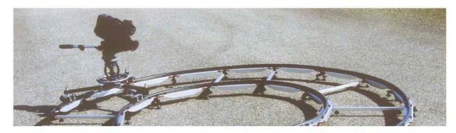
For situation that the dolly is not used for a longer time period it is recommended to place the dolly at one of the end positions on the Track. This prevents the situation that temporary bumps of the wheels are causing disturbing image movements.
