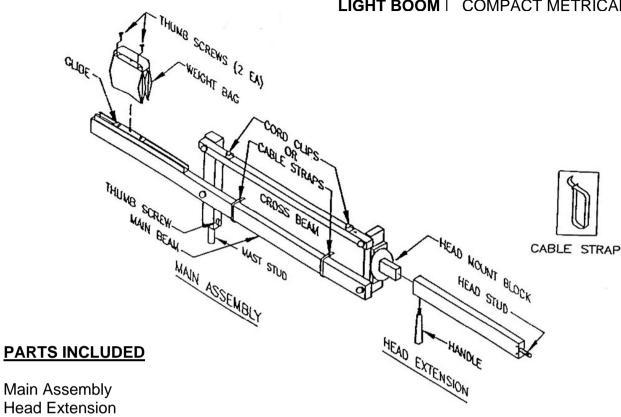
Main Assembly Head Extension Head Stud Handle Cord Clips (2) Cable straps (2) Weight Bag
