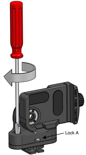
Flip the holder 90° by pressing the "lock A", please tighten the second screw.
