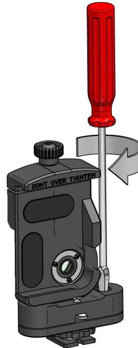
First tighten the right screw using a flat screw driver or a long Allen key (3mm)
