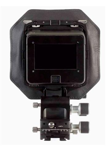
The Actus-DB features a convenient lens stop that limits the quick sliding movement. This serves two functions. First you can set the infinity distance of your lens as a reference point and second it protects the rear element from touching the sensor of the digital back.
