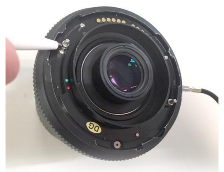
The pin indicated with the pencil needs to be in this position. The shutter will be closed, but after setting it to T you can open it with a cable release. After that it can remain open and you'll be able to use the aperture ring.
